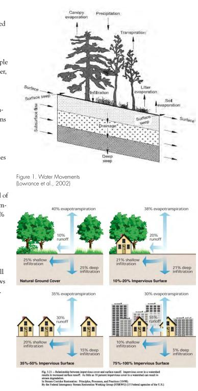
Figure 2. Relationship between impervious cover and runoff (FISRWG
